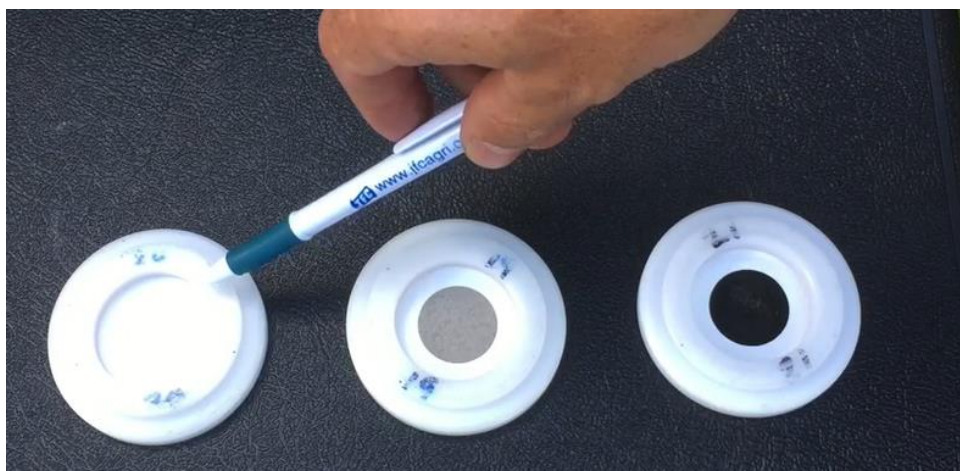
Figure 1. Example of 3 different pollution filters used in professional stations for monitoring the air quality. Photo from the EPA Ireland video ( link )
